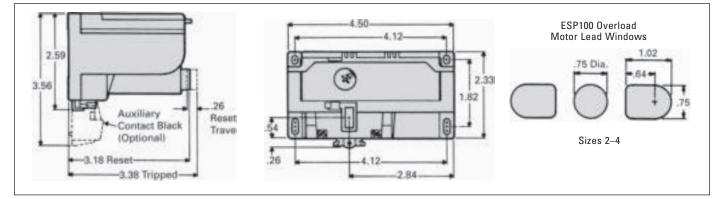
Note: Dimensions for reference, not for construction. Dimensions in inches.
